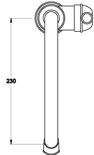
Note: Mixer requires a Ø35mm hole in bench or basin Max benchtop thickness of TBA
