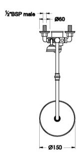
Note: G ½" BSP female fittings required in the wall (B) Fixed center, taps must have 150mm centres (A) Maximum, adjustable, can be reduced at installation
