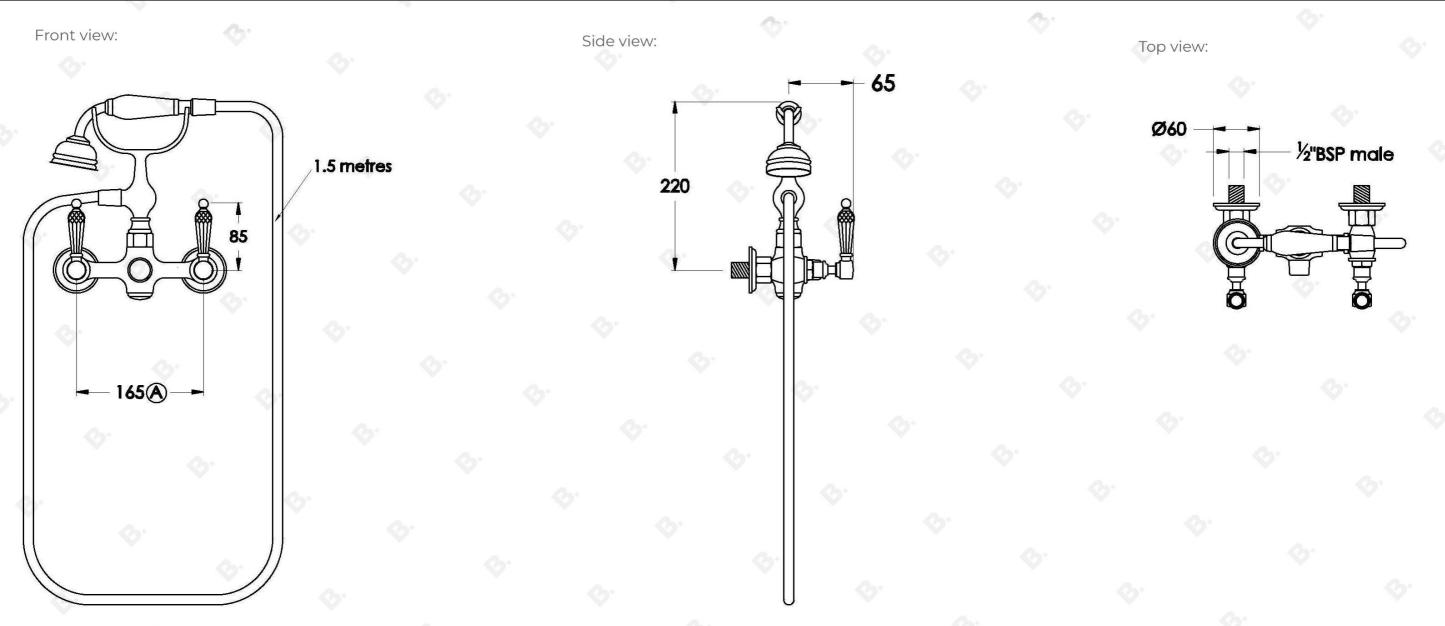
Note:  $G_2^1$  BSP female fittings required in the wall (A) Fixed centre; outlets must have 165mm centres
