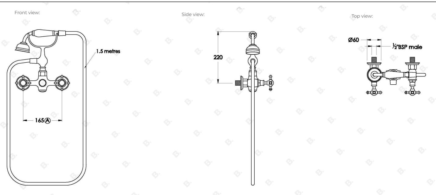
Note:  $G_2^1$  BSP female fittings required in the wall (A) Fixed centre; outlets must have 165mm centres
