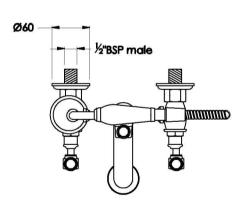
Note:  $G\frac{1}{2}$  "BSP female fittings required in the wall A Fixed centre; outlets must have 165mm centres
