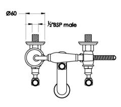
Note: G½" BSP female fittings required in the wall (A) Fixed centre; outlets must have 165mm centres
